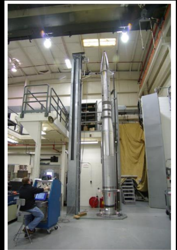
Figure 6.2.5-1: Bend Test Fixture at WFF
