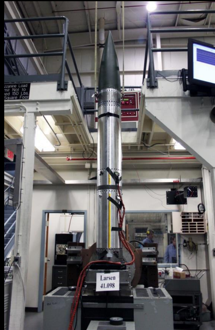
Ling Electronics B335 Thrust Axis Shaker at WFF
