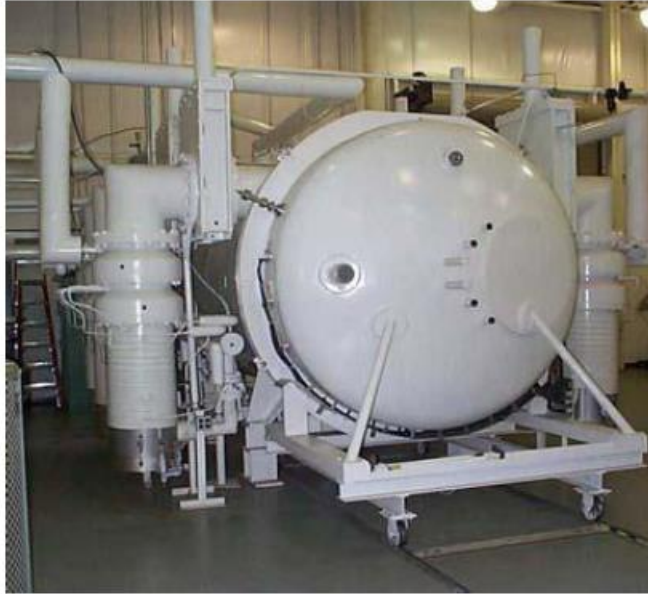
Figure 6.2.4-1 PV/T Vacuum Chamber (left) and Tenney Space Simulation System Thermal Vacuum Chamber at WFF
