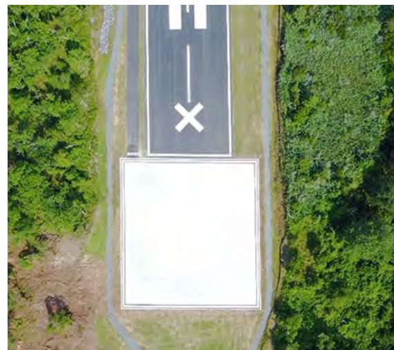
Figure 74: Concrete vertical takeoff and landing (VTOL) Pad rated to 5,000 psi
