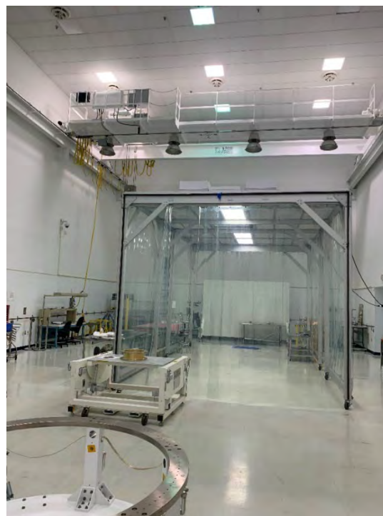
Figure 58: High Bay East Cleanroom Tent with ESPA ring integration ground support equipment in the foreground
