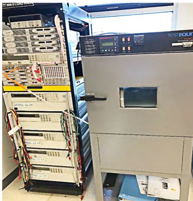
Figure 12: Test Equity Model 115 Thermal Cycle Chamber
